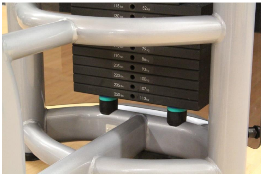
Figure 6 Impact Absorbers to Resistance Equipment
